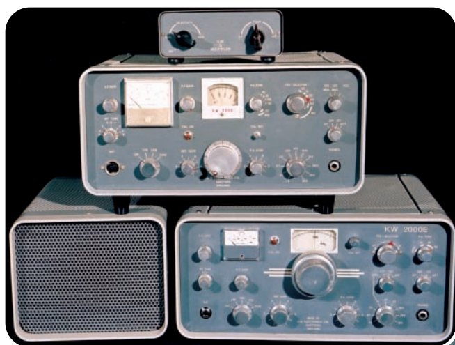
● Fig. 1: The original KW2000 mounted above the later KW2000A, power supply unit (with integral speaker) on the left and Q Multiplier on top.
