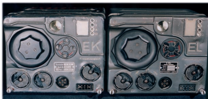
● Fig. 5: The German E10K, left, and E10L receivers. Simple controls are tuning, volume and beat frequency oscillator (b.f.o.) on/off. The 4 pin socket on the lower front is the headphone jack.
