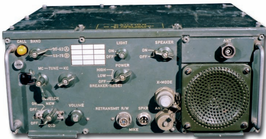
● Fig. 3: The RT-524 Low band v.h.f. Transceiver, (slight modification to the microphone socket but otherwise original).
