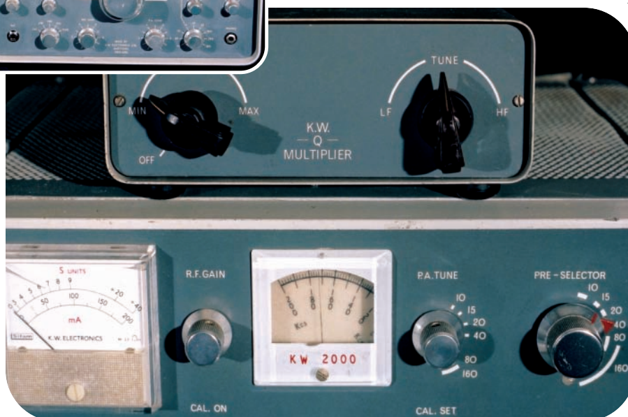
● Fig. 2: Close up of the KW Q Multiplier, a single transistor is used in this model.
